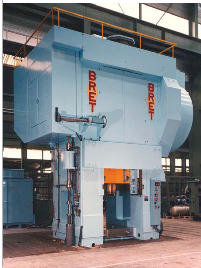
Presse de forge 4 500 tonnes. 4 500-ton forging and die stamping press.
