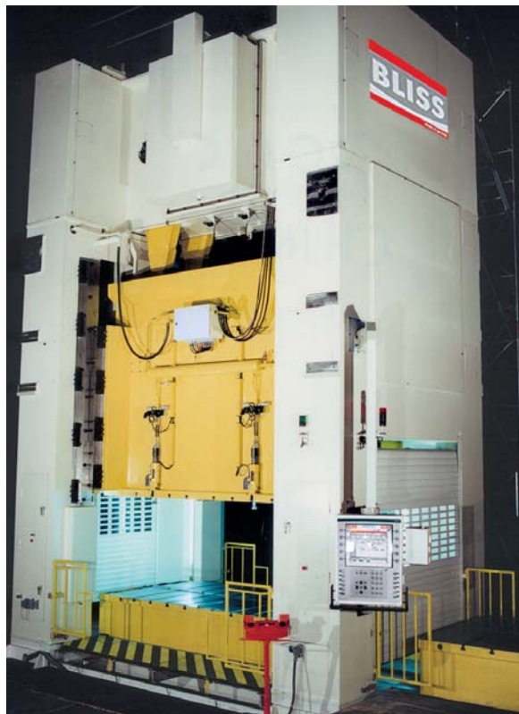
600-ton, 4 point, 2 rolling bolsters mono directional G1 type drawing press.
